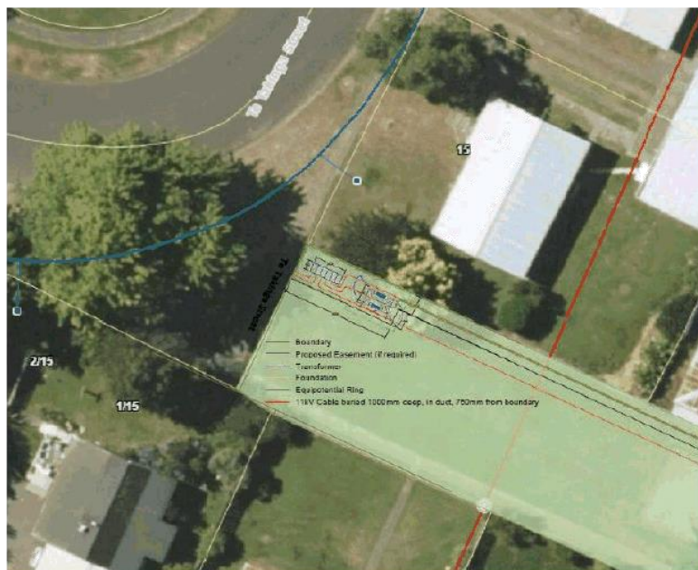
Proposed location of equipment within reserve. (Scale is correct)
