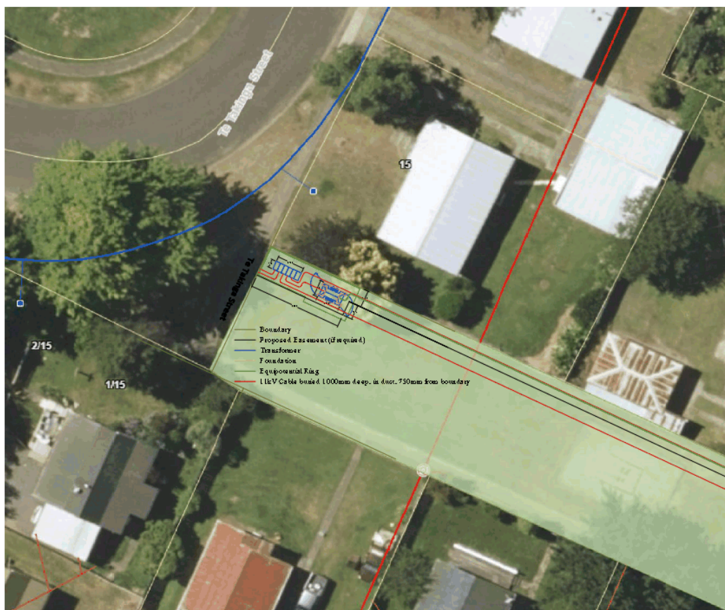
Figure 2 - Location of proposed transformer, high voltage switch and cables in reserve
