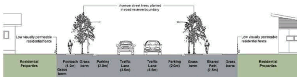
Figure 9-F: Cross section of Collector and Secondary Collector Roads in the General Residential Zone
