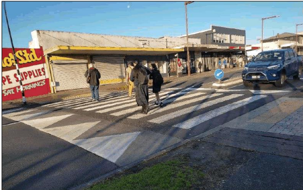
Figure 5 Raised platform priority crossing
