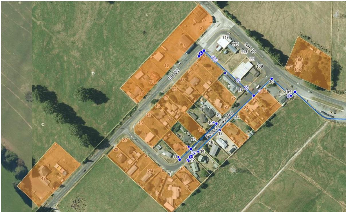
Image 1: Orange Highlighted properties are not currently connected to water. Blue lines identify the existing water mains
