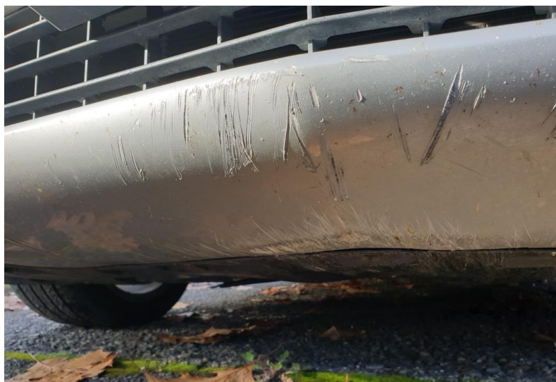
Above. Scouring of bumper from scraping on lifted concrete.
