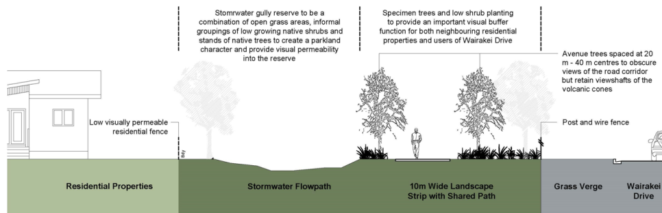
Figure 9-A: Cross section illustrating the Wairakei Drive road frontage design
