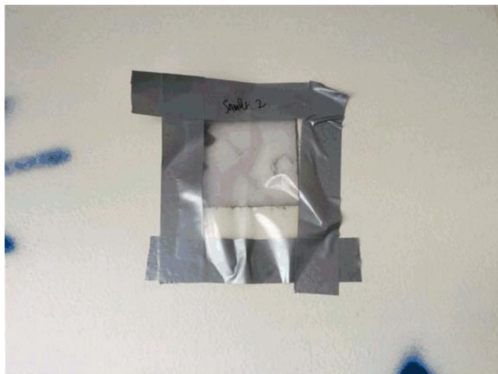
Zone 2- Insulating Board Secondary Wall Linings - Confirmed ACM
