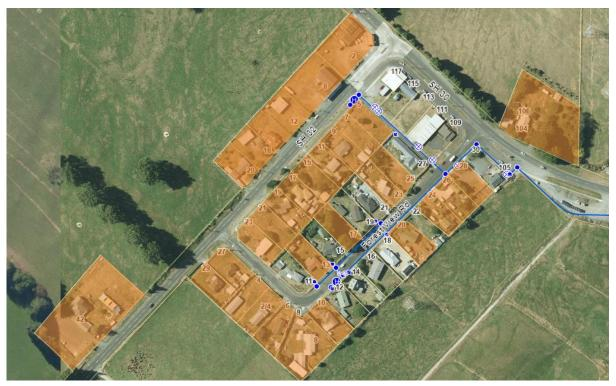
Image 1: Orange Highlighted properties are not currently connected to water. Blue lines identify the existing water mains
